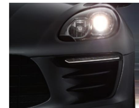
Dipped beam with halogen headlights
