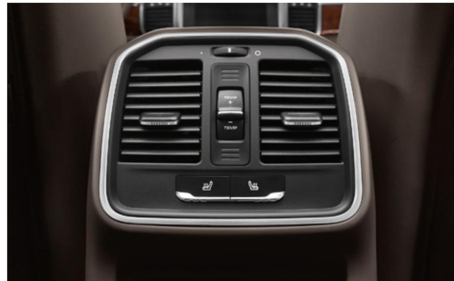
Climate control buttons in rear for three-zone automatic climate control
