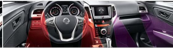
Fully automatic air conditioning with dual zone, temperature sensor and digital display
