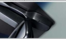
Rain sensing and automatic light control unit
