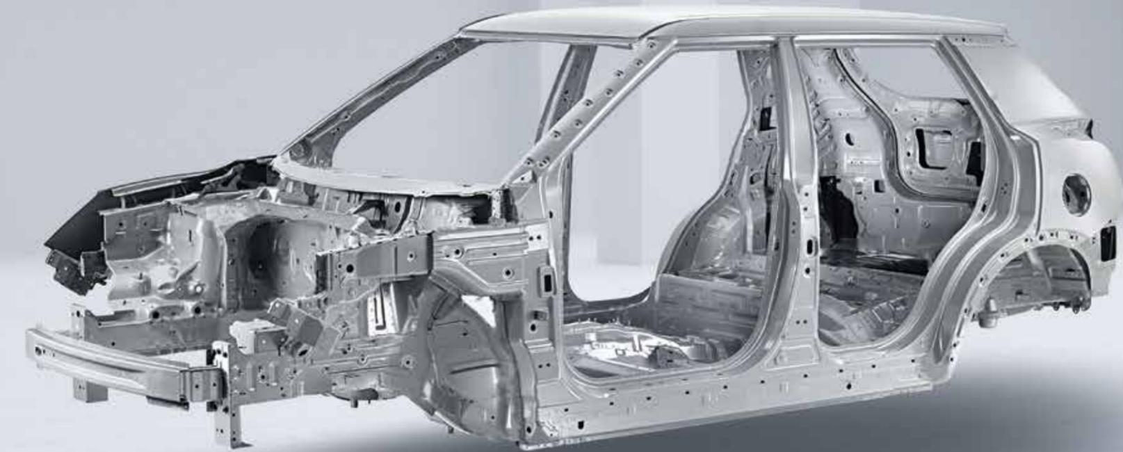
Extensive use (71.4%) of high tensile-strength steel plate minimises frame deformation in a collision for maximum protection of vehicular occupants.
