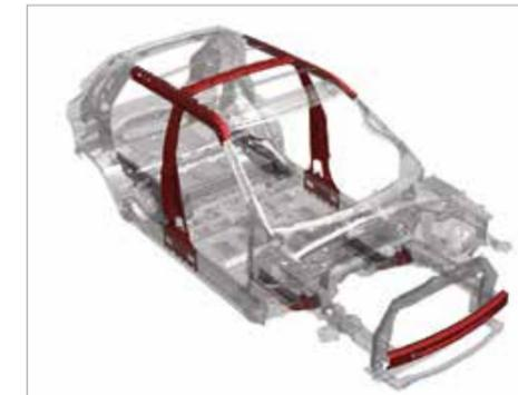
Ultra-high-tensile steel plate at ten key points in the frame to further enhance occupant safety.
